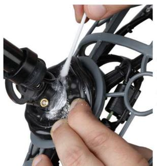
After use in salty or dusty environments, the bellows may become sticky, that's why from time to time it is advisable to clean it with soap and water to avoid rubbing noises and add a little talc baby powder where the parts can touch, specifically in and around the bellows hole.
