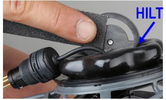
14- if necessary, sand the surfaces in contact between the hilt and the swivel base for a better tightening of the base during use (100 grit sandpaper)
