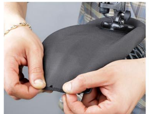
15- after use in dusty or salty environments, the bellows may become sticky, it's advised to clean it with soap+water and put some baby talc powder around and in the bellows hole to avoid rubbing noise.
