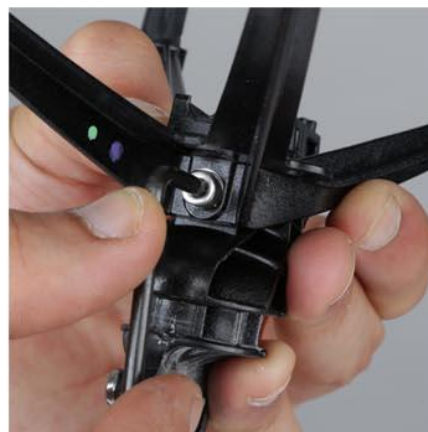
8- with a hexa key 3mm separate the hilt from the cross
