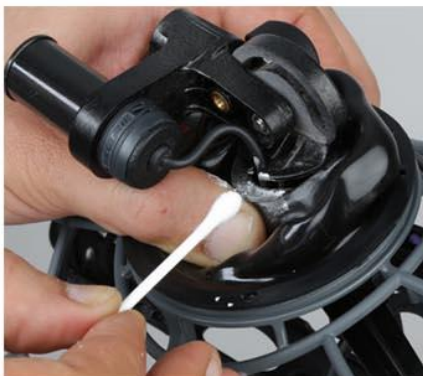
15- after use in dusty or salty environments, the bellows may become sticky, it's advised to clean it with soap+water and put some baby talc powder around and in the bellows hole to avoid rubbing noise.
