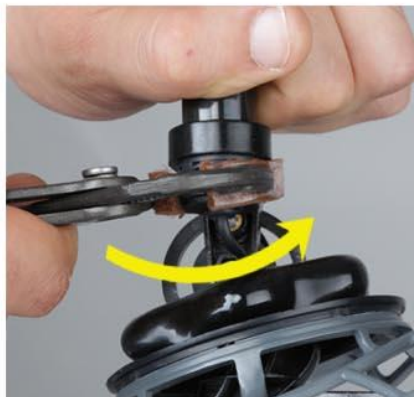
2- unscrew the XLR's boot holding the metal body fixed
