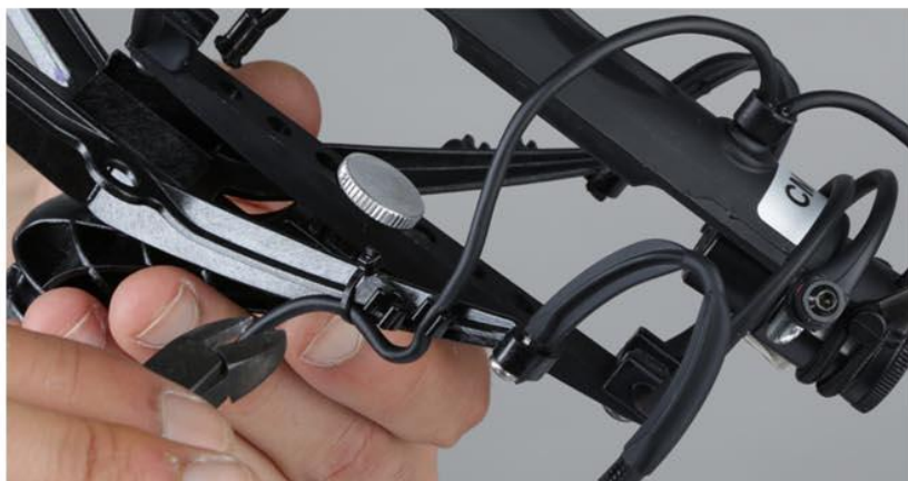
7- cut the tie-rip, detach the cable and unscrew the suspension module
