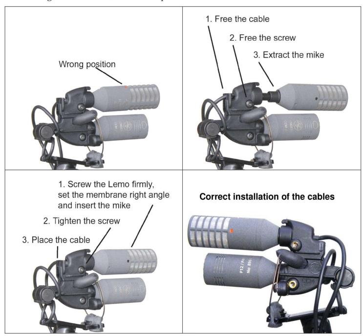
**Note**: The side screw has to be tightened quite firmly. Always screw or unscrew it with the microphone in position.
