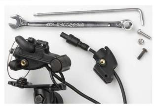
5- Side (S) cable installation: Unscrew the two M3 screws in order to release the upper part of the module to pass the cable through, then replace this module, the M3x12 screw + nut is only used to secure the fixation.
